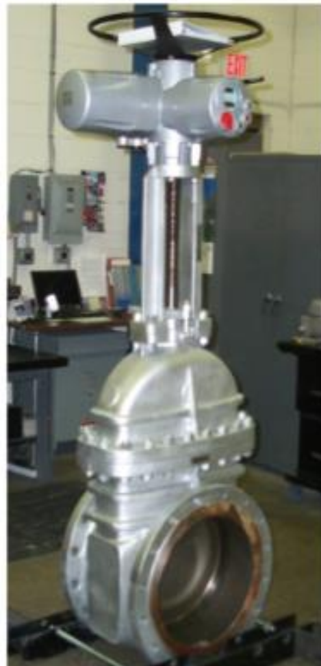
Fig. 3. BIFFI ICON 2000 electric actuator fitted onto a disassembled valve.
