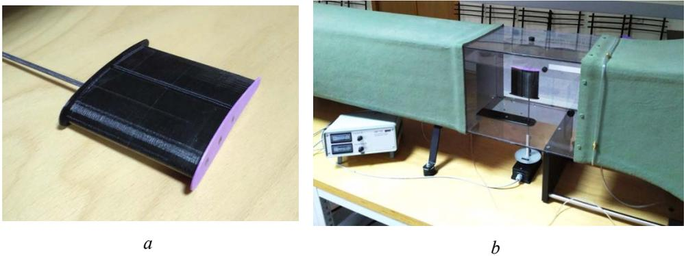
**Fig. 7.** Experimental setup: *a* - blade segment model, *b* - blade segment mounted in the wind tunnel.
