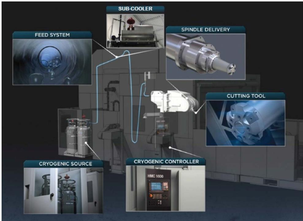
**Fig. 1.** Example of cryogenic system from 5ME Company [43]
