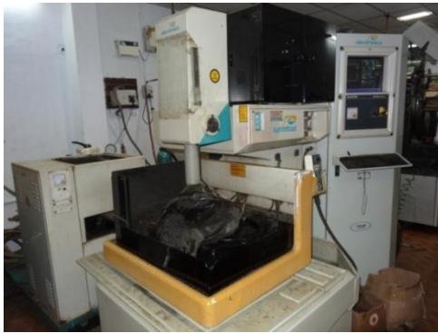
Fig. 1 WEDM experimental set up (Electronica Sprint cut)
