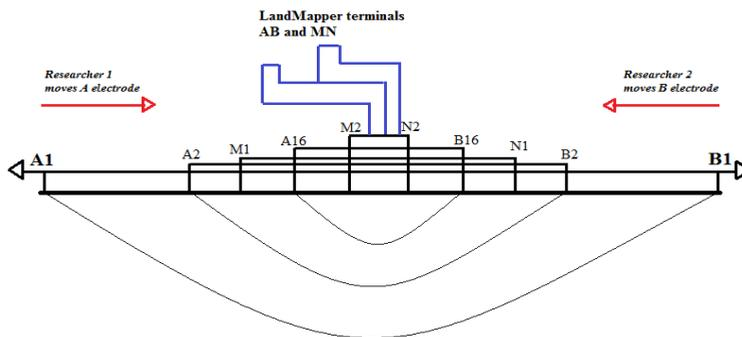
**Fig 2.** Schematic representation of Schlumberger geometry and with using of LandMapper device.
