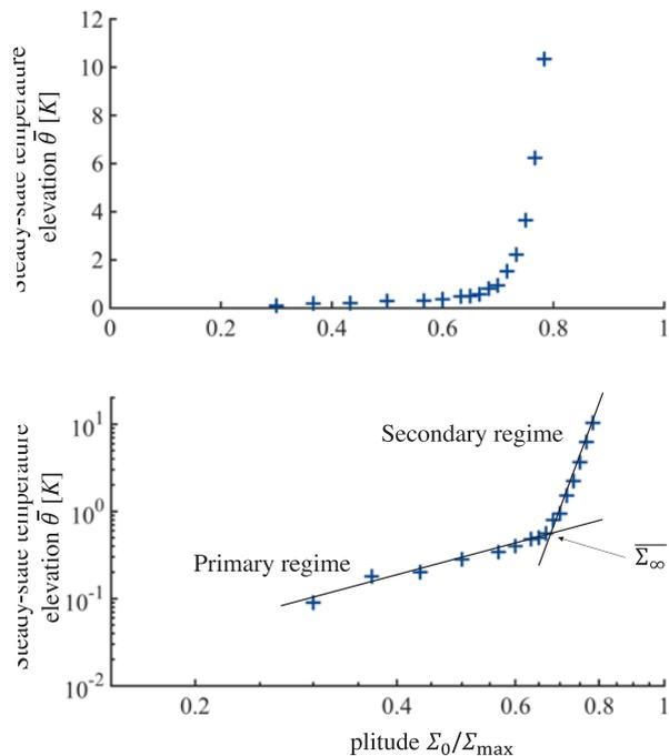
**Fig. 5.** Self-heating curve for the condition  $T=250^{\circ}C$  and  $R=-1$ .
