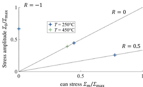
Fig. 10. Haig diagram obtained by self-heating measurements.
