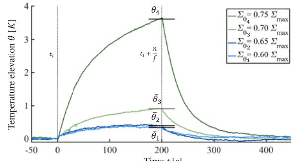
**Fig. 4.** Evolution of the mean temperature elevation during several blocks of cyclic loadings.
