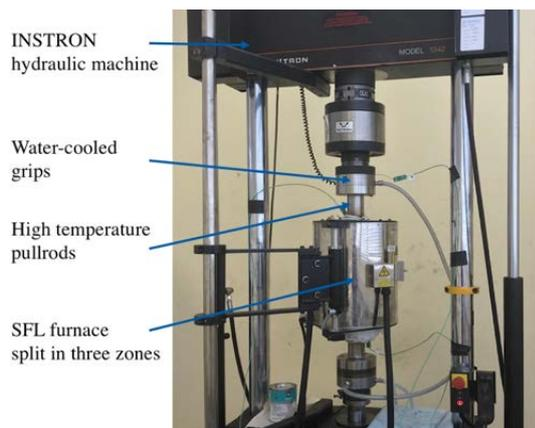
**Fig. 1.** Experimental device for the self-heating test at high temperature.
