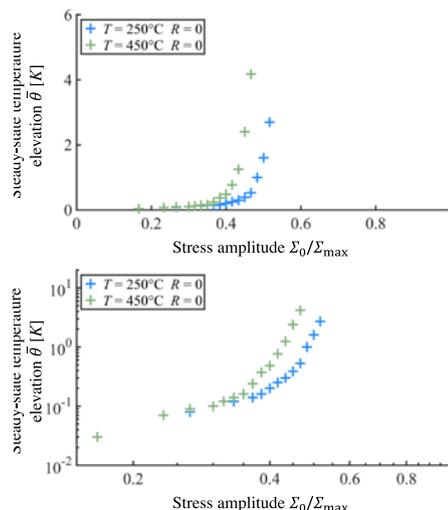
**Fig. 7.** Influence of the temperature on the self-heating curves for the loading ratio  $R=0$ .
