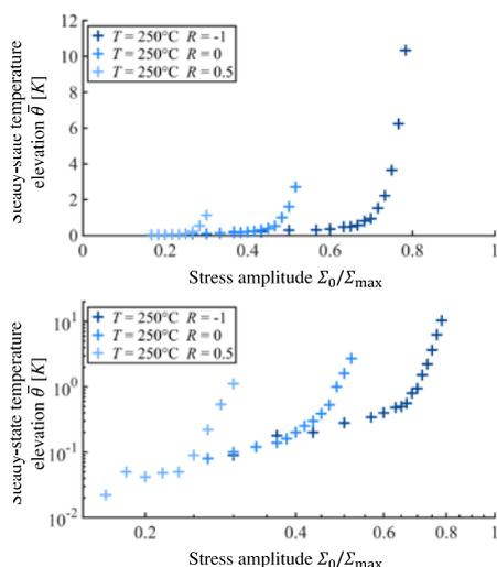
**Fig. 6.** Influence of the loading ratio  $R$  on the self-heating curves for the temperature  $T=250^{\circ}\text{C}$ .
