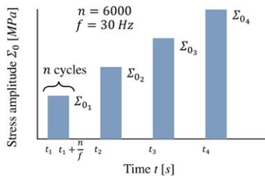
**Fig. 3.** Successive series of cyclic loadings with increasing stress amplitudes.
