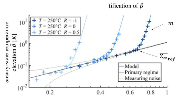
**Fig. 9.** Analysis of the self-heating curves and identification of the model parameters.
