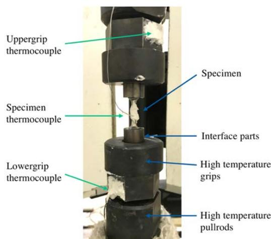
**Fig. 2.** Geometry of the specimen and thermocouples fixing.
