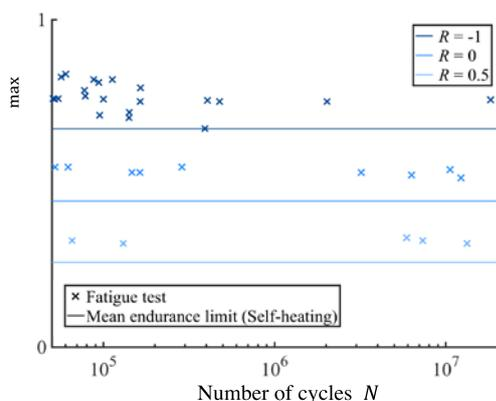
Fig. 11. Comparison of mean endurance limits obtained by the self-heating method with classical fatigue tests at  $250^{\circ}\text{C}$ .
