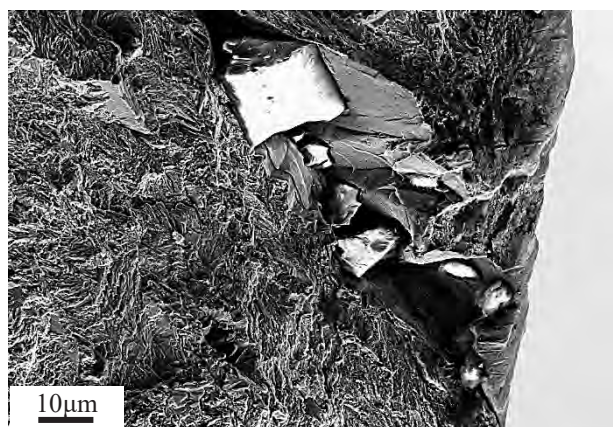
Fig. 15. Fractography of failed TWIP3.0 sheared and sandblasted sample, showing the fatigue initiation site.
