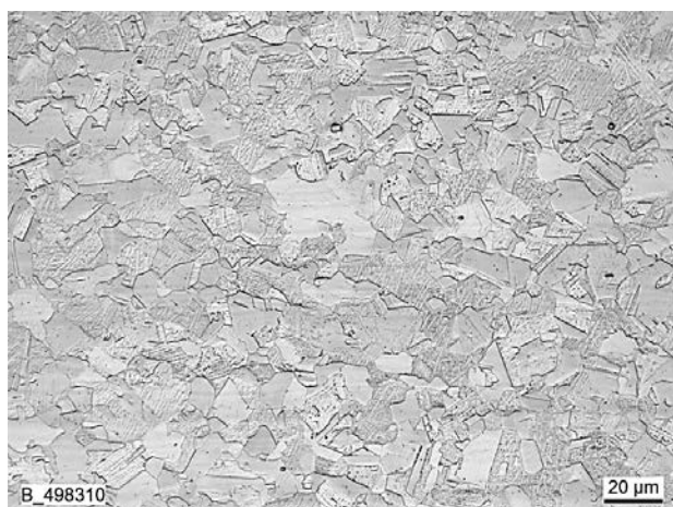
Fig. 2. Microstructure of TWIP3 at the centre (Wallner etched).
