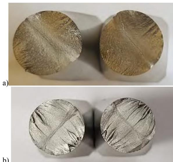
**Fig.6.** An example test piece photo taken after oscillatory bending test a) 6082-T6 b) 2017(A)-T4
