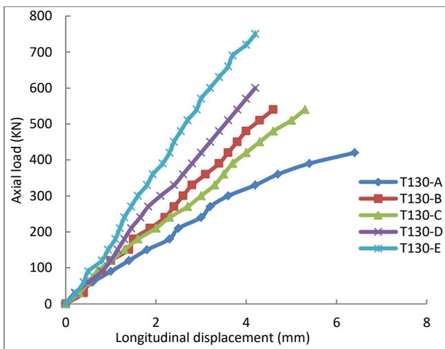
**Fig.16.** Load-longitudinal displacement curves for CFRP confined tied columns with internal tie spacing 130 mm.
