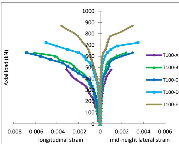
**Fig.12.** Load- strain curves for confined CFRP tied columns-T100
