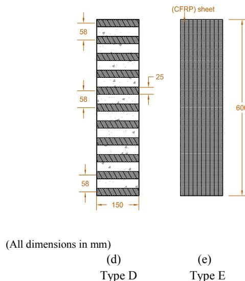
**Fig .2.** Types of CFRP confinement.
