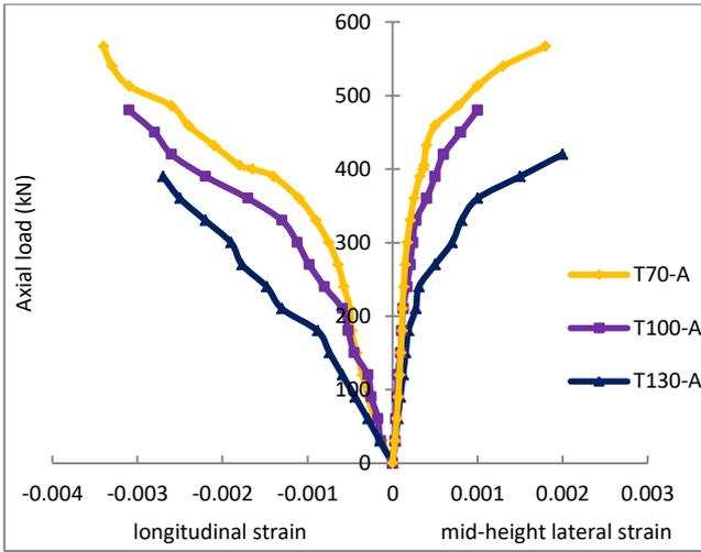
**Fig. 10.** Load- strain curves for unconfined CFRP tied columns.
