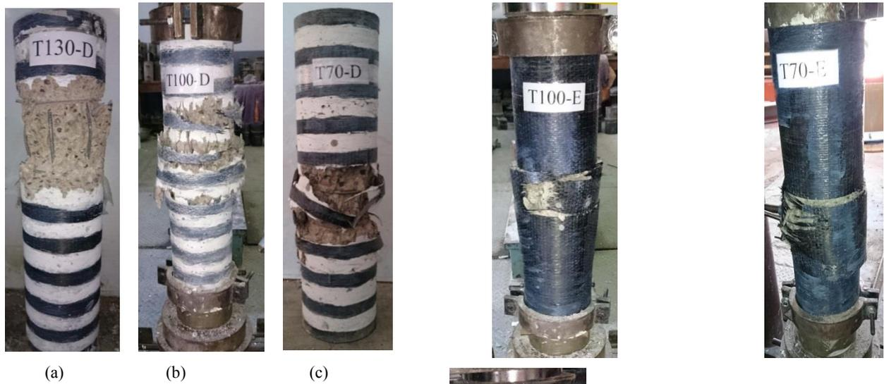
**Fig 8.** Failure modes for columns type (D)
