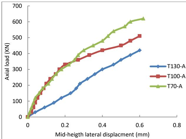
**Fig.15.** Load-lateral displacement curves for un-confined tied column.
