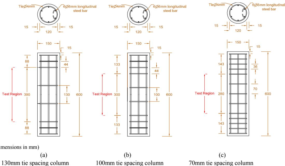
**Fig .1.** The geometry of the tied column specimens.
