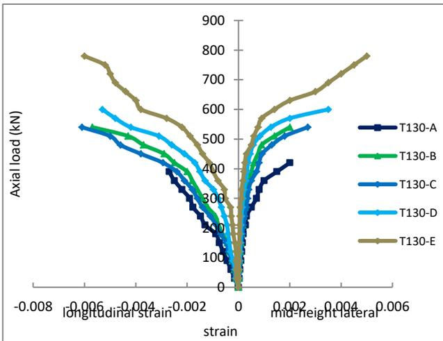
**Fig.11.** Load- strain curves for confined CFRP tied columns-T130.
