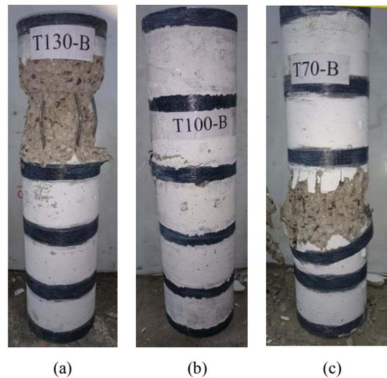
**Fig 6.** Failure modes for columns type (B)
