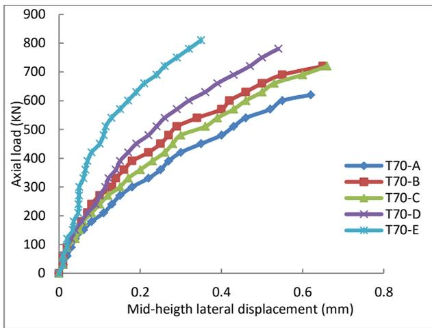
**Fig.21.** Load-lateral displacement curves for CFRP confined tied columns with internal tie spacing 70 mm.
