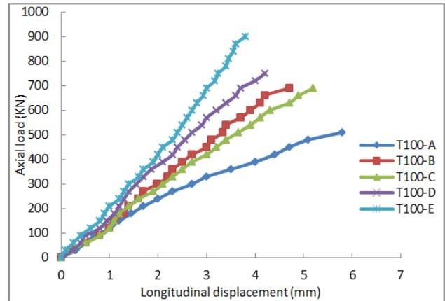
**Fig.17.** Load- longitudinal displacement curves for CFRP confined tied columns with internal tie spacing 100 mm.
