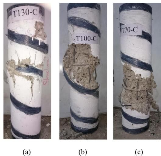
**Fig 7.** Failure modes for columns type (C)
