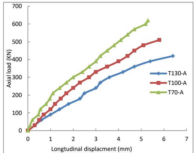
**Fig.14.** Load- longitudinal displacement curves for un-confined tied column.
