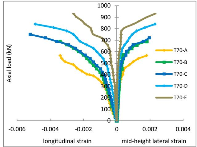
**Fig.13.** Load- strain curves for confined CFRP tied columns-T70.
