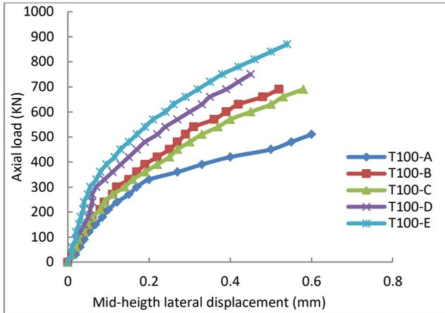
**Fig.20.** Load-lateral displacement curves for CFRP confined tied columns with internal tie spacing 100 mm.
