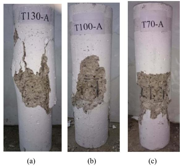
**Fig 5.** Failure modes for control columns
