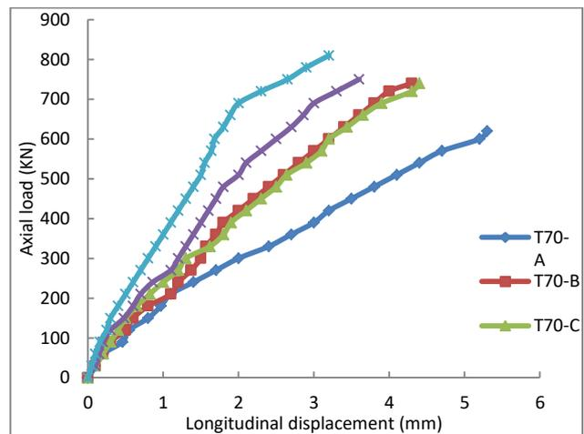
**Fig.18.** Load-longitudinal displacement curves for CFRP confined tied columns with internal tie spacing 70 mm.
