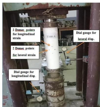
**Fig. 4.** Locations of dial gauges and demec points for the column specimen.
