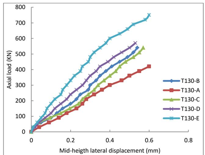
**Fig.19.** Load-lateral displacement curves for CFRP confined tied columns with internal tie spacing 130 mm.
