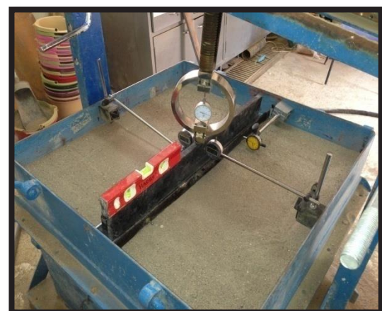
Plate (4): A steel plate model which transfer distributed line load on the strip footing.
