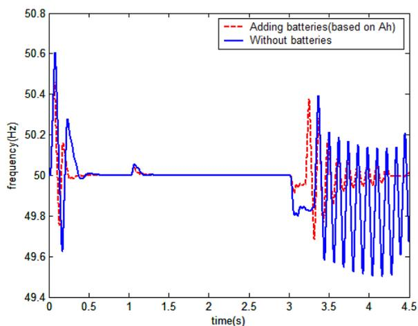
**Figure 9.** Frequency variation of power grid after adding sodium sulfur battery (based on Ah)
