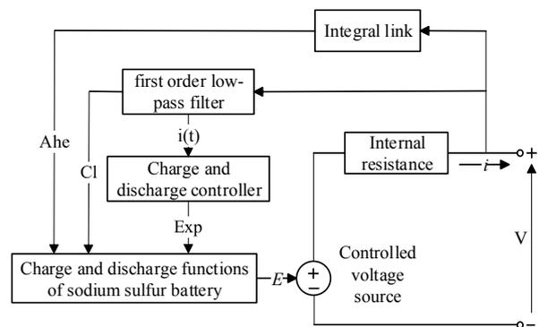
**Figure 1.** The circuit model of battery
