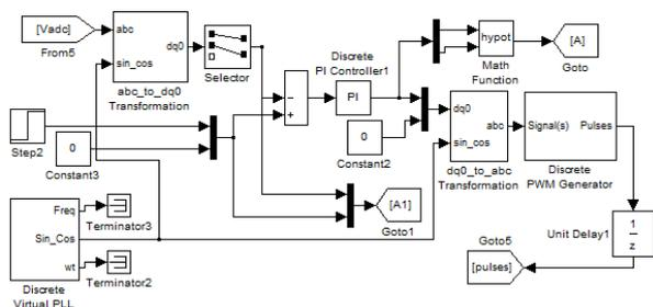
**Figure 6.** Inverter control circuit
