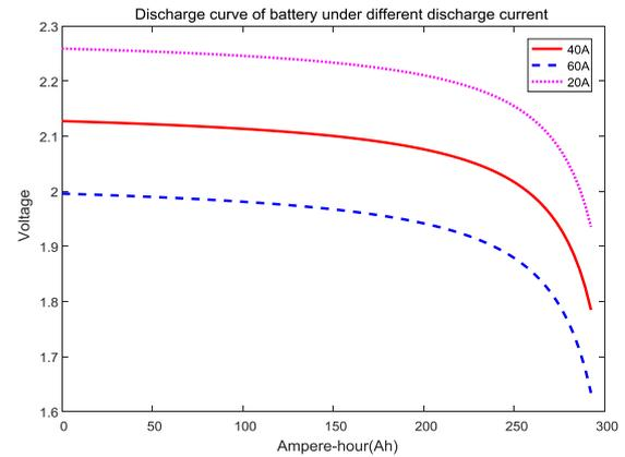
**Figure 2.** The discharge curves under different current.
