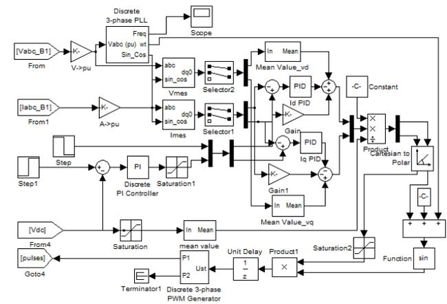
**Figure 5.** Rectifier bridge control circuit
