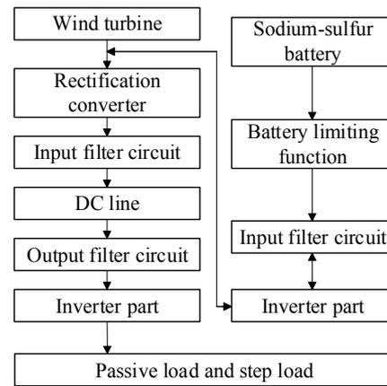
**Figure 4.** AC/DC power transmission model
