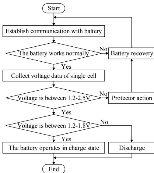
**Figure 7.** Control strategy with battery voltage as the standard
