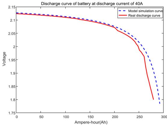
**Figure 3.** The discharge curves under 40A
