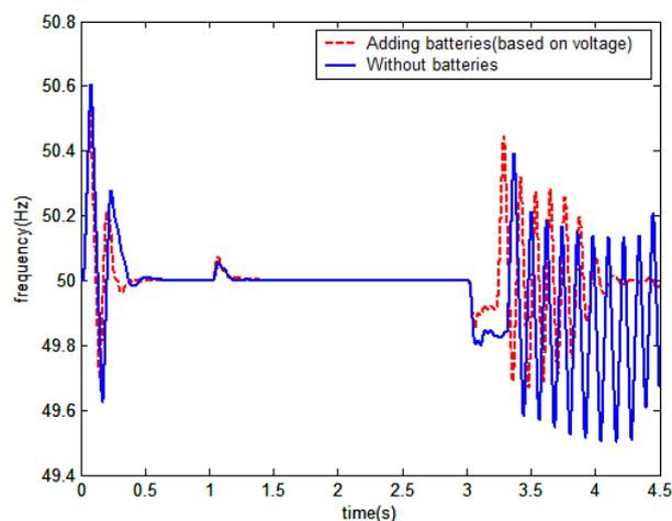
**Figure 8.** Frequency variation of power grid after adding sodium sulfur battery(based on voltage)
