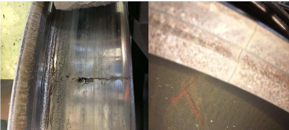
**Fig. 9.** Damaged wheel [14]
