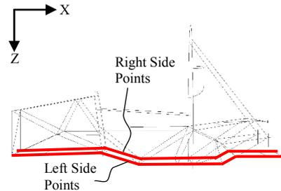
**Figure 5.** Data points location on the frame.
