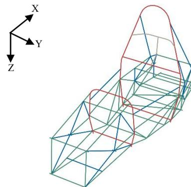
Figure 1. Tubular frame FE model.
