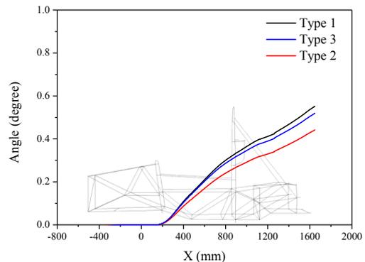
**Figure 7.** Frame torsional angle curve (Mode II).
