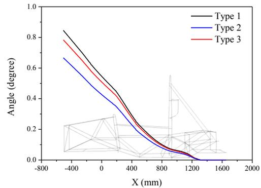
**Figure 6.** Frame torsional angle curve (Mode I).
