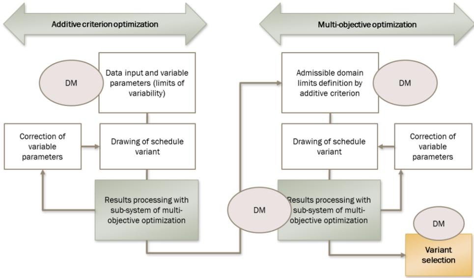
**Fig. 2.** Technology of schedules generation with the help of an IDSS
