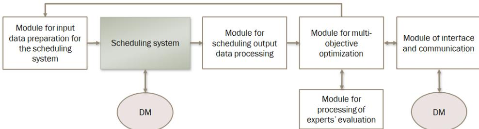
**Fig. 1.** Architecture of IDSS for scheduling under the conditions of multi-objective optimization
