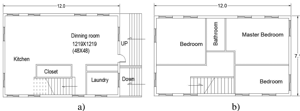
Fig. 1. Floor plan of the single-family detached house: a) first floor; b) second floor. Dimension in m.
