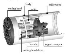
Fig. 1. Mechanized tunnel shield
