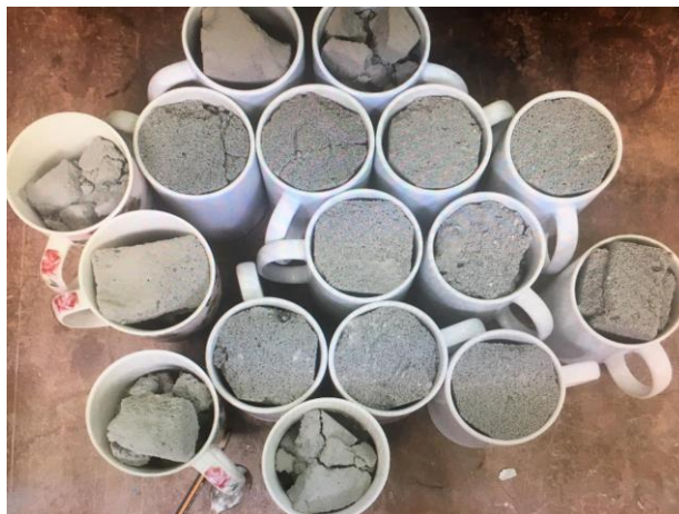
Fig. 3. The fragments of samples in the molds before placing in a drying oven
