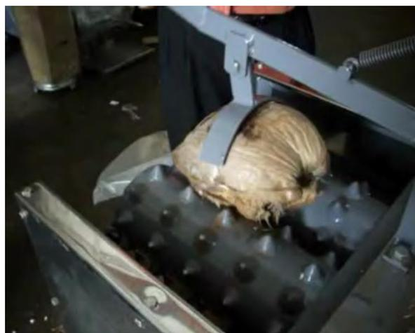
**Fig. 2.** A horizontal roller dehusking machine [2].
