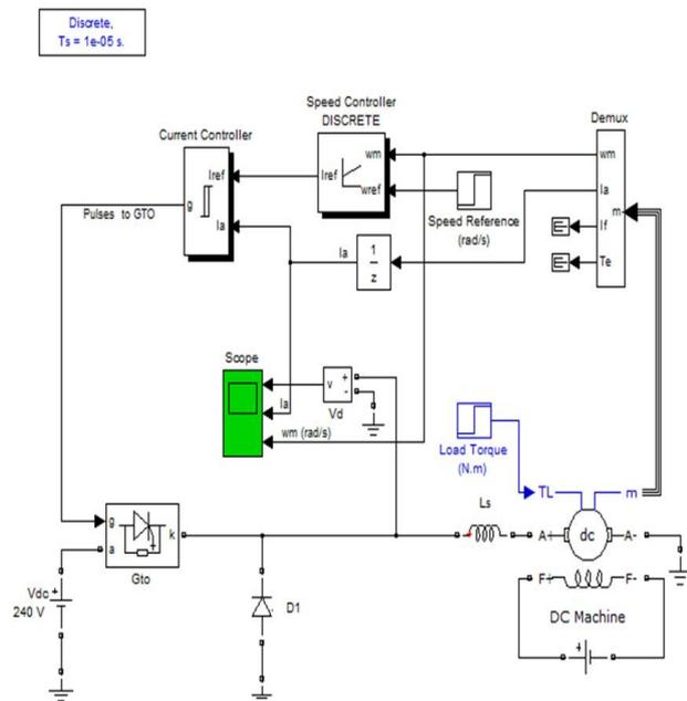
Fig. 4. A DC motor model in Simulink.
