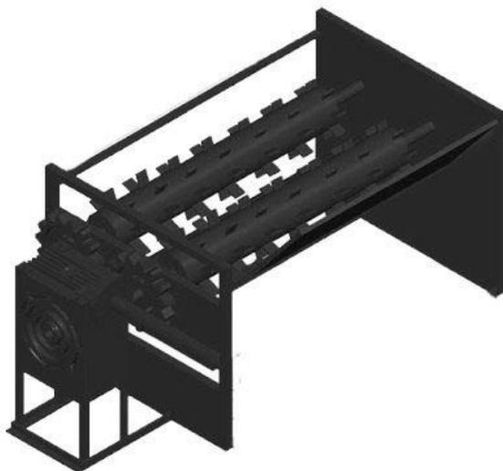
**Fig. 9:** Solar PV coconut dehusking machine model.
