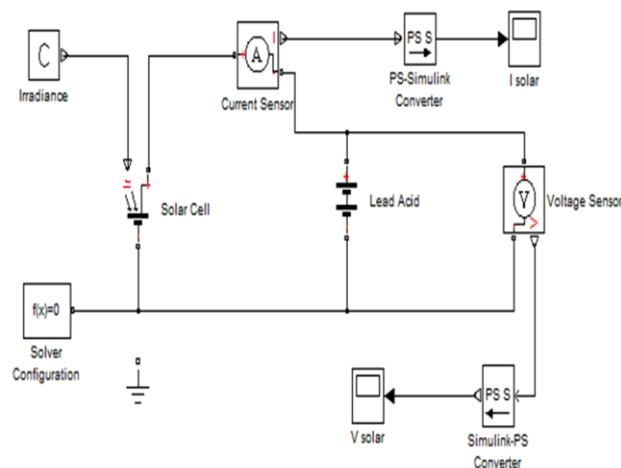
**Fig. 3.** A solar cell model in Simulink.
