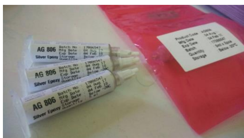
Fig. 4. Silver-epoxy based ink (Model: AG806)
