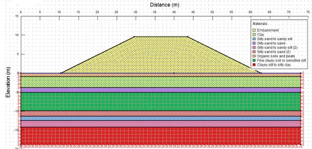
**Figure 6 :** The component layers of the PK 116 + 720 survey
