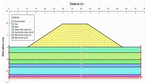
**Fig.5.** The component layers of the PK 116 + 580 survey
