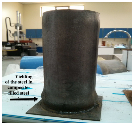
b) Failure mode
