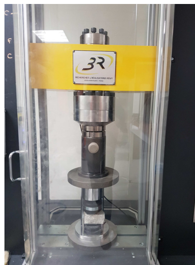
Fig. 2. Compressive strength testing machine
