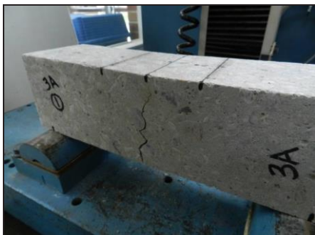
Fig. 15. Crack propagation and widening after the ARS reloading phase.
