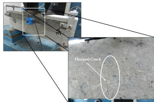
Fig. 14. Typical flexural crack following the ARS initial loading phase.
