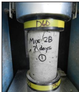
Fig. 7. Typical failure. Fig. 8. Exposed GeoTech matrix after failure.
