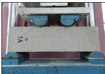
Fig. 5. BFRC flexural specimen in the loading apparatus.
