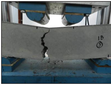
Fig. 11. Typical failure of flexure specimen.
