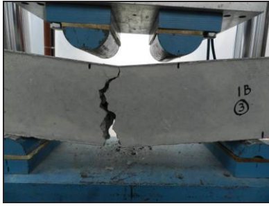
Fig. 11. Typical failure of flexure specimen.
