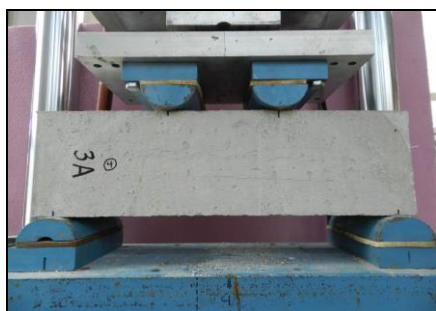
Fig. 5. BFRC flexural specimen in the loading apparatus.
