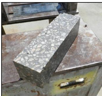
Fig. 4. ARS specimen after cutting.
