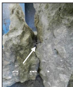
Fig. 7. Typical failure. Fig. 8. Exposed GeoTech matrix after failure.
