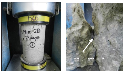
Fig. 7. Typical failure. Fig. 8. Exposed GeoTech matrix after failure.
