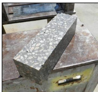
Fig. 4. ARS specimen after cutting.
