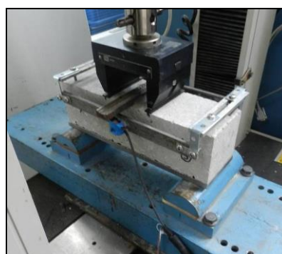
Fig. 6. ARS setup for the initial loading phase.
