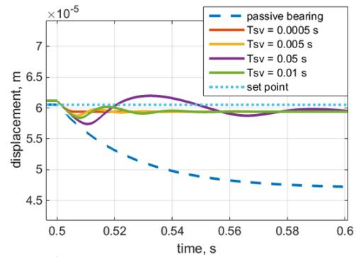
**Fig. 8.** Trajectories of the rotor depending on the time constant of a servo valve.
