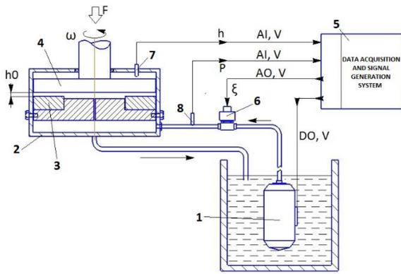
Fig. 1. Conceptual model of an AHTB.
