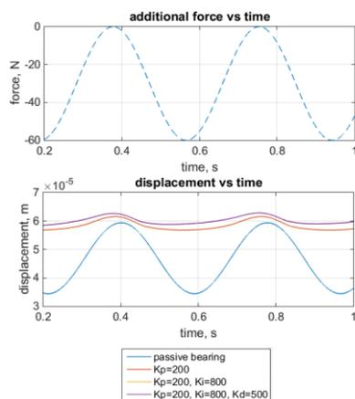
**Fig. 9.** Trajectories of the rotor on an AHTB under periodic load
