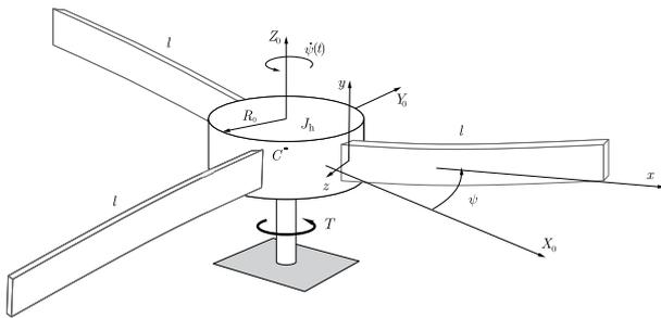
**Figure 1.** Model of the rotating hub with three elastic beams
