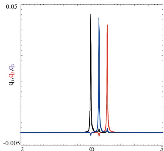
**Figure 2.** Resonance curves for amplitude of excitation  $\rho = 0.01$  of displacements of each beam, beam No.1 - black line, beam No.2 - red line and beam No.3 - blue line
