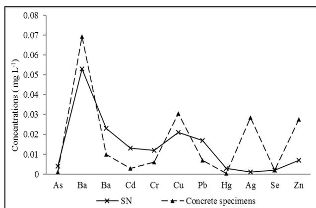
**Fig. 2.** Comparison of TCLP analysis of concrete specimen and nickel slag.
