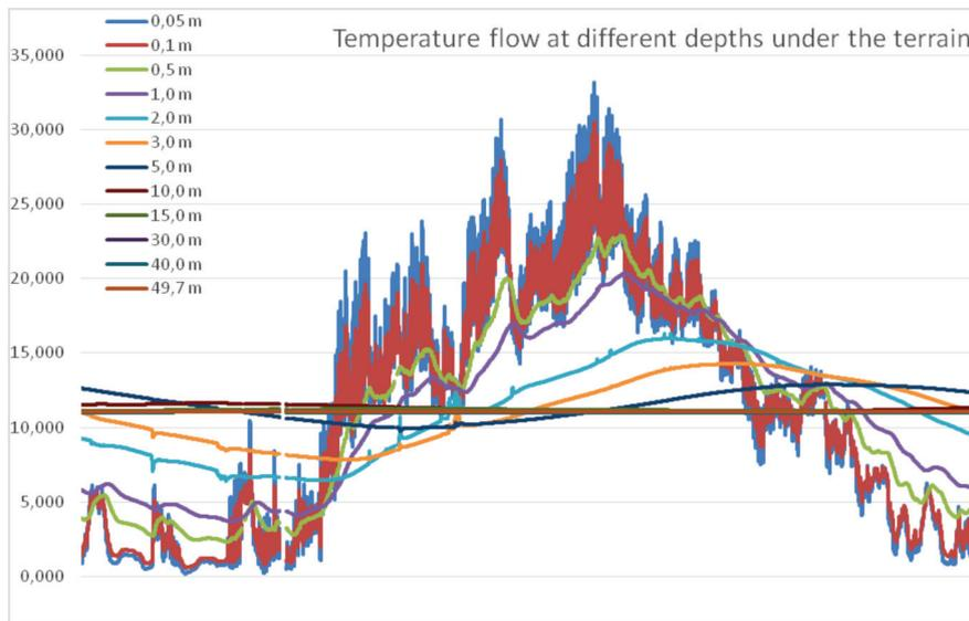
**Fig. 2.** Temperature flow at different depths under the terrain.
