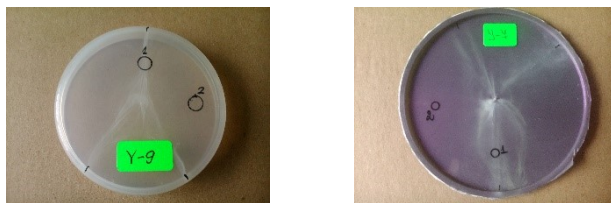
Fig 1. Disposition of visual defects on the injection moulded products
