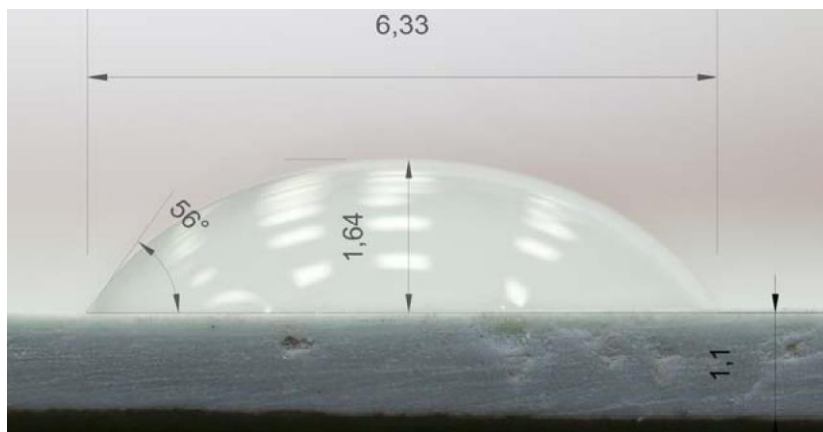
Fig. 7. Photograph of a drop on the horizontal surface of the protective material Subcote FLP with the edge angle 56^\circ
