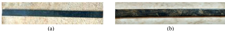
Fig. 2. Fabricated Specimens for Tensile Test as per ASTM Standards (a) Woven Flax and Sisal Fiber Reinforced Composite; (b) Randomly oriented Flax and Sisal fiber reinforced composite
