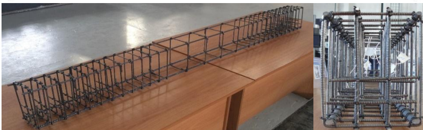
Fig. 3. The scheme of reinforcement of concrete structures under study: 1 – reinforcement Ø6 mm grade A240; 2 – reinforcement Ø10 mm grade A500; 3 – reinforcement Ø5 mm grade Bp500; 4 – equal leg angle 100×10mm.
