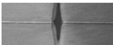
Fig. 8. Laser welded TRIP joint specimen after tensile test
