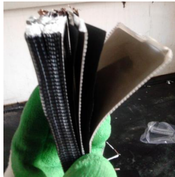
Fig. 2. The positive of the overcharge battery.
