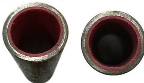
Fig. 1. Polyethylene lined tubing samples
