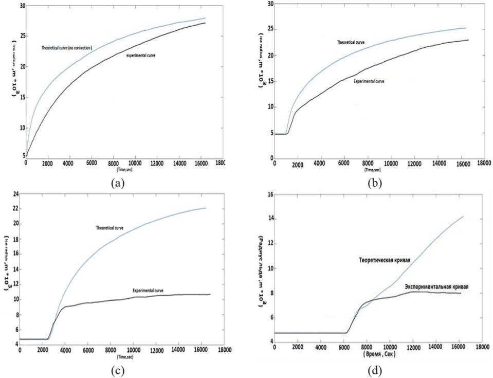
**Fig. 2.** Theoretical (without convection) and experimental ice radius versus time at different heights (22, 17.5, 15, 12.5) cm with (a, b, c, d) consequently.
