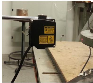
Fig. 4. Laser displacement sensor.
