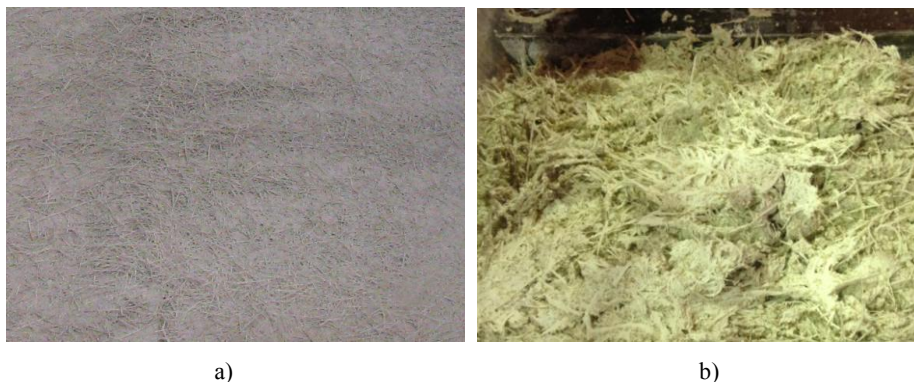
Fig 4. Alignment of fiber filaments obtained from a) sprayed technique and b) premixed technique
