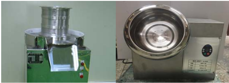
Fig. 1 Manufacture of capsules (capsule core fabricating equipment ; left, Wall material coating equipment ; right)
