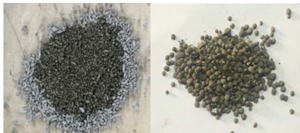
Fig. 8 Qualitative evaluation of wall material coating (before coating ; left, after coating ; right)
