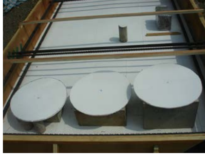
Fig. 1. Photo of defects buried in the specimen.
