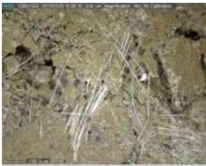
Fig. 5. Crack pattern in fibrous geopolymer concrete due to tensile load.
