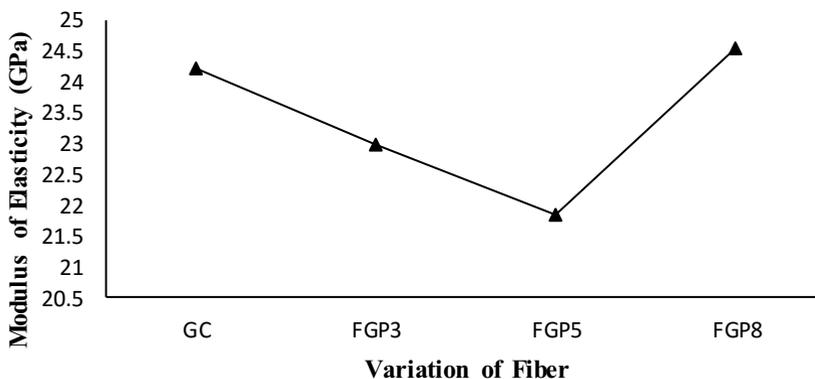
**Fig. 7** Modulus of elasticity due to fiber variations.
