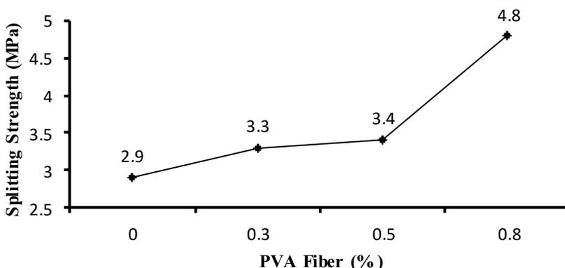
**Fig. 3.** Splitting strength caused PVA fiber variations.
