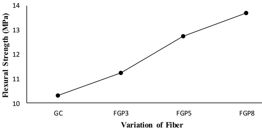
Fig. 6 The effect of fiber adding to flexural strength.
