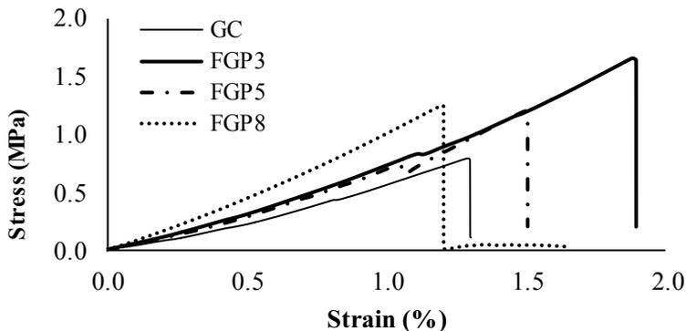
Fig. 4. Stress – strain diagram of direct tensile test.
