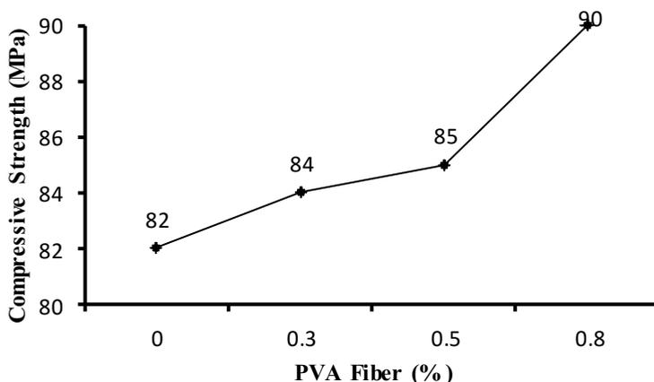
**Fig. 2.** Contribution of fiber variations to compressive strength.
