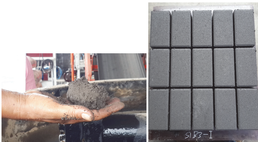
Fig. 1. Water required to make a stiff mixture and the paving specimens produced.
