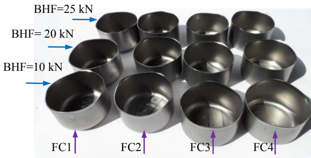
Fig. 2. Representative deep-drawn cups resulted from different combinations of friction conditions (FC) and blank-holding forces (BHF).
