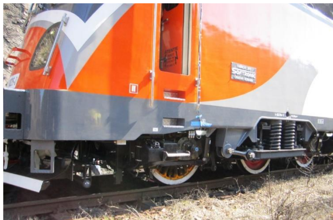
Fig. 3. LE-MA 26 equipped with the measuring wheelset during the on-track tests
