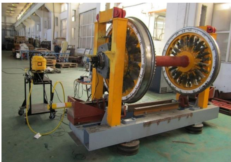
Fig. 1. Calibration stand with measuring wheelset mounted for the calibration procedure
