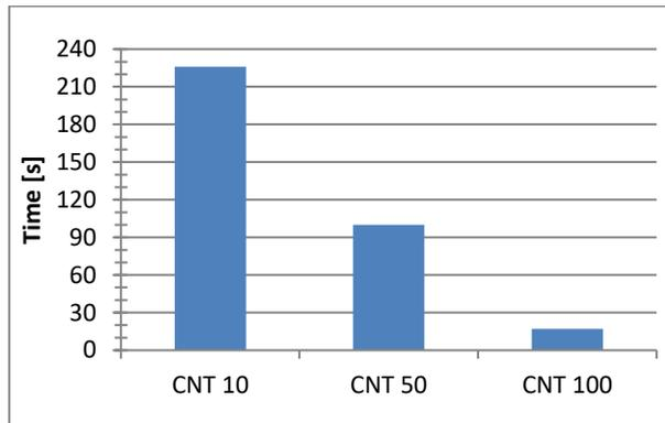
**Fig. 3** The effect of the CNT parameter on the time required to execute two circular paths in one direction.
