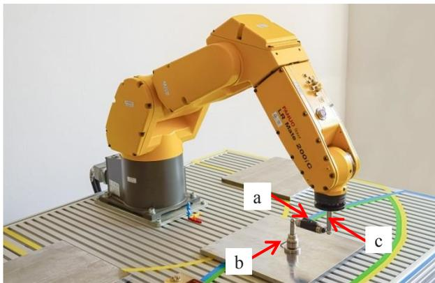
**Fig. 1.** Measuring assembly: a-Ballbar, b-magnetic center pivot, c-magnetic tool cup.
