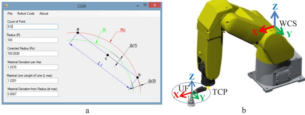
**Fig. 2** Application for calculate points on the circle (a) and position of the coordinate systems on the Fanuc LR Mate 200iC robot (b).
