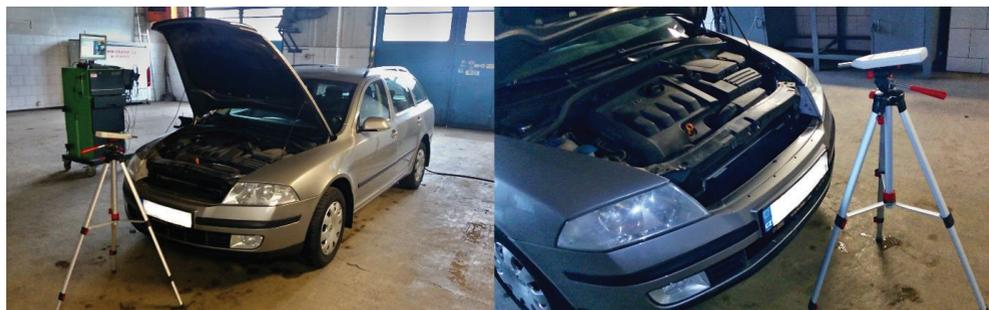
**Fig. 1.** Measurement of engine noise. Source: authors
