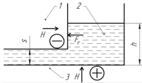
**Fig. 2.** The forces acting on the workpiece on the machine table: 1 – workpiece; 2 – rheological ferromagnetic liquid; 3 – machine table
