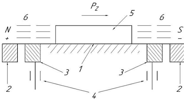
**Fig. 1.** Scheme of workpiece positioning on magnetic table: 1 – magnetic table; 2 и 3 – magnets; 4 – controllers of magnetic field force; 5 – workpiece; 6 – rheological ferromagnetic liquid
