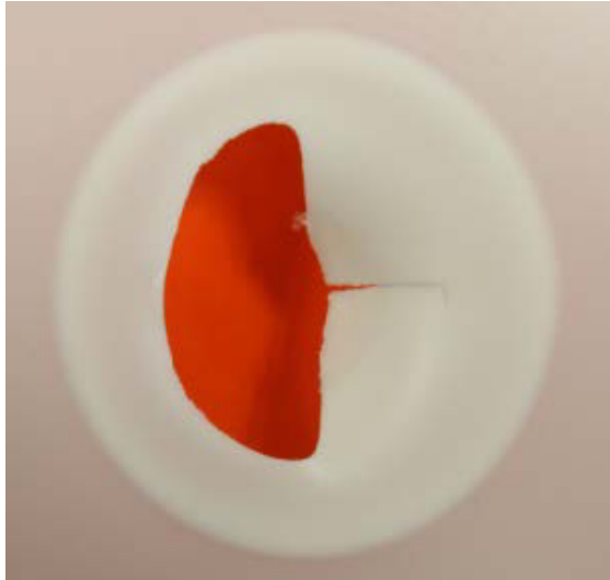
Fig. 6. HIPS deformation after drop weight test at 100 J.
