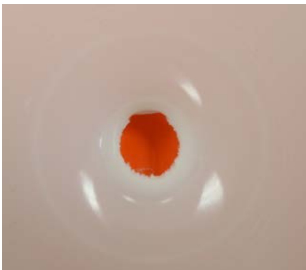
Fig. 9. HDPE deformation after drop weight test at 230 J.
