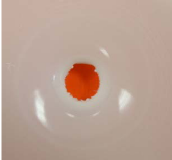
Fig. 7. HDPE deformation after drop weight test at 150 J.
