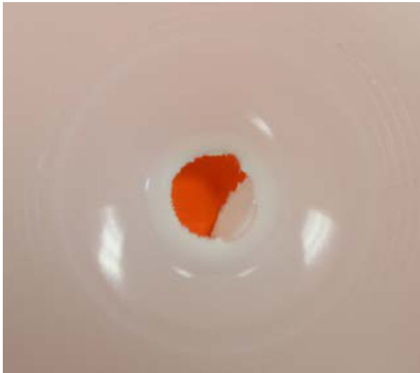
Fig. 8. HDPE deformation after drop weight test at 200 J.
