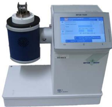
**Figure 7.** Mettler Toledo DMA1
