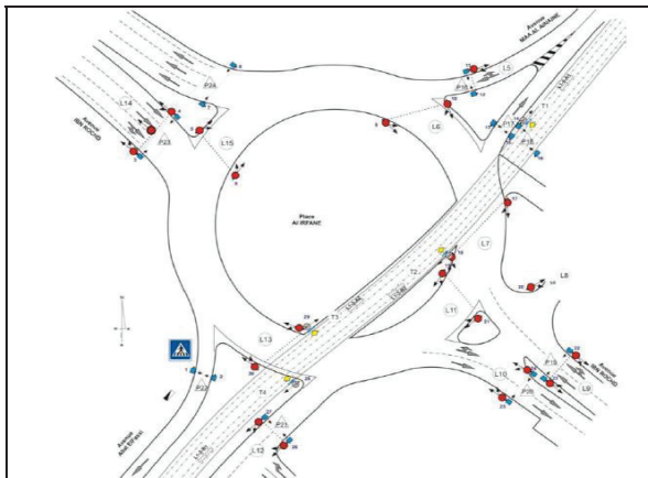
Figure 2. The layout of the signalized roundabout under study “IBN ROCHD Roundabout” is a tram roundabout with four arms. The configuration is following: two lanes going into intersection and one separate lane for vehicles to turn right. Diagram of intersection geometry is in figure2.
